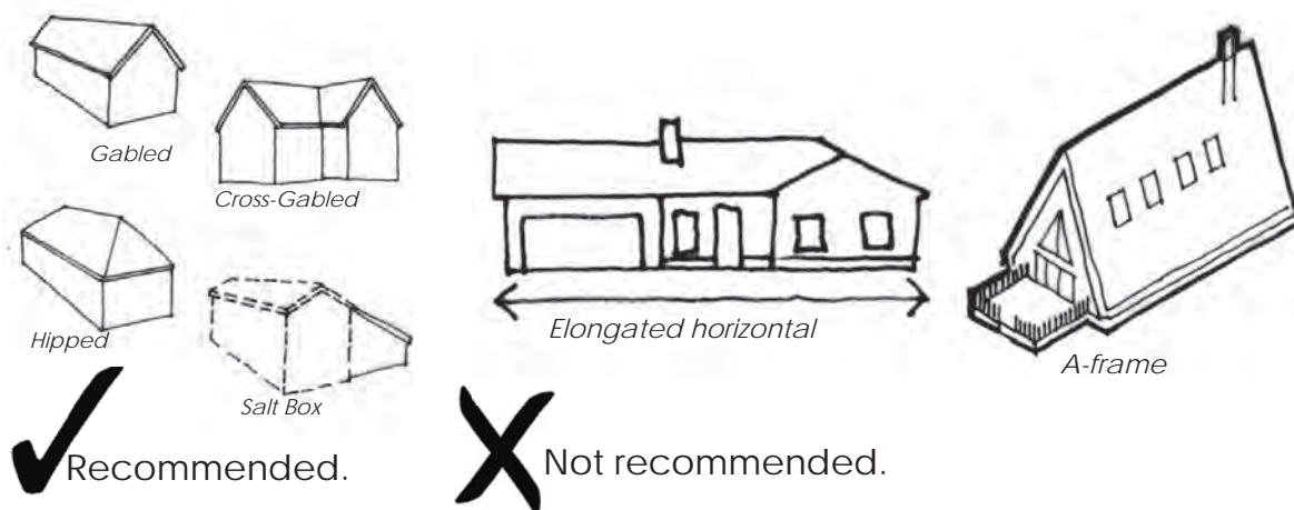
Figure 3-9. Design new buildings so that they reflect local historic building forms and shapes, whether gabled, cross-gabled, or hipped. Avoid forms such as elongated ranch styles and A-frames. Source: JMA collection.
