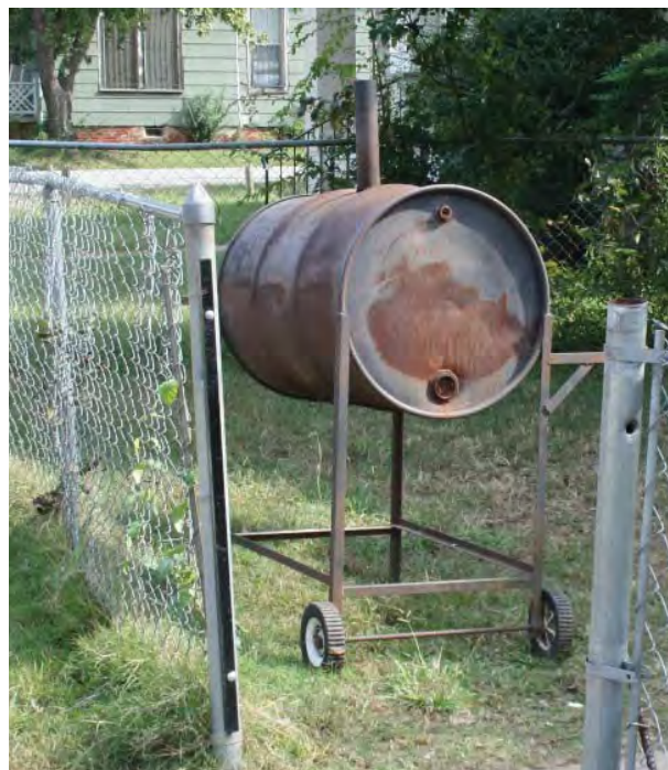
Figure 2-167. Backyard smoker fabricated from an oil drum. Source: John Milner Associates, Inc., 2007.
