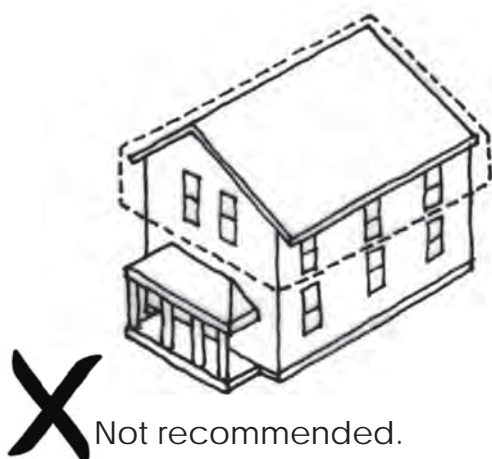
Figure 3-3. Place additions to existing buildings to the rear of the building, instead of “building up. Consider adding a connector to set off the historic part of the building and to make the addition more easily removable. Source: JMA collection.
