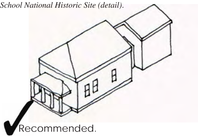
Figure 3-3. Place additions to existing buildings to the rear of the building, instead of “building up. Consider adding a connector to set off the historic part of the building and to make the addition more easily removable. Source: JMA collection.
